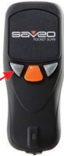
Press and hold for 3-4 seconds to unpair from device.
