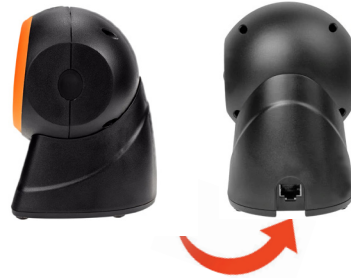
Power and Data cable input
